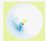
BinWaves: disaggregation of the full directional wave spectrum monochromatic into bins. simulation with SWAN to derive propagation coefficients (Kp), and superposition of bins to reconstruct nearshore spectra
